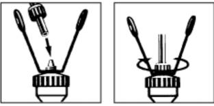
Place a nut, thread outwards, onto the end of the tube. Push Hanger Strap over filter top. Push the tube onto the tapered end of the filter top as far as it will go. Tighten the nut firmly. Repeat at the Saddle Connector end.
