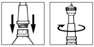
Insert the black valve unit into the top of the cone, valve downwards. Before inserting the valve into the top of the cone, check to ensure the top and bottom caps (part nos 412767
