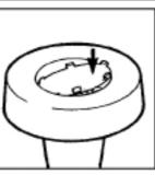
Remove all components from carton. Fill the recess in the underside of the black ballast bowl with ballast or sand, up to just below the holes at the top of the recess (3lbs or 1.36kilos). Place the ballast retaining lid (with six lugs uppermost) into the ballast recess, fitting two adjacent lugs into their recesses. Then press each of the remaining four lugs home working round in a clockwise direction.
